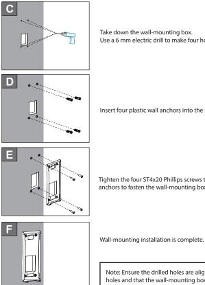
Take down the wall-mounting box. Use a 6 mm electric drill to make four holes.
