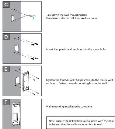
Insert four plastic wall anchors into the screw holes.
